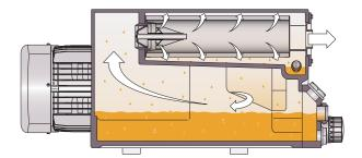
The machine works on the rotary vane principle.
