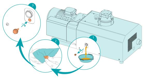
For oil type and oil capacity see *Technical Data*  $[\rightarrow 31]$  and Oil chapters.
