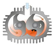
The machine works on the claw principle.
