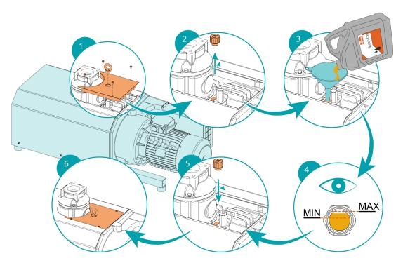
The oil level should stay constant over the lifetime of the oil. If the level does fall, this indicates a leak and the machine requires repair.
