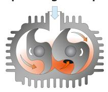
The machine works on the claw principle.
