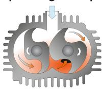
The machine works on the claw principle.
