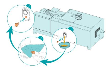
For oil type and oil capacity see *Technical Data*  $[\rightarrow 28]$  and *Oil*  $[\rightarrow 30]$ .
