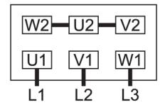
Double star connection, multi-voltage motor with 9 pins (low voltage):
