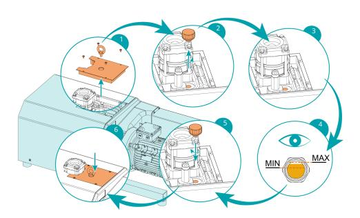
The oil level should stay constant over the lifetime of the oil. If the level does fall, this indicates a leak and the machine requires repair.
