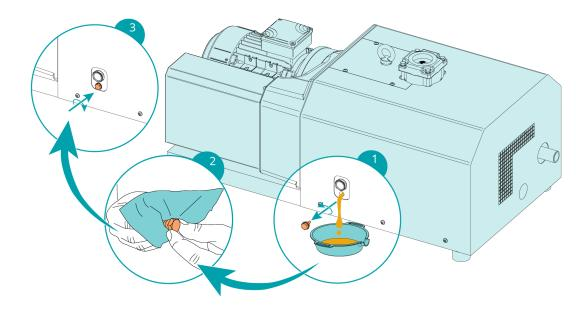
For oil type and oil capacity see *Technical Data* [ $\rightarrow$  28] and *Oil* [ $\rightarrow$  30].
