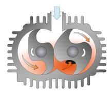
The machine works on the claw principle.
