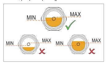
If the oil level does not reach the target circle level:
