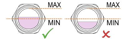
• Fill up if necessary, see Filling Cooling Liquid [→ 18].
