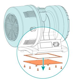
Star connection (high voltage): 380-415 V (50 Hz), 380-480 V (60 Hz) Factory default setting Delta connection (low voltage): 190-220 V (50 Hz), 200-240 V (60 Hz)
