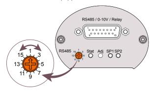
The communication is effected via serial interface RS485:
