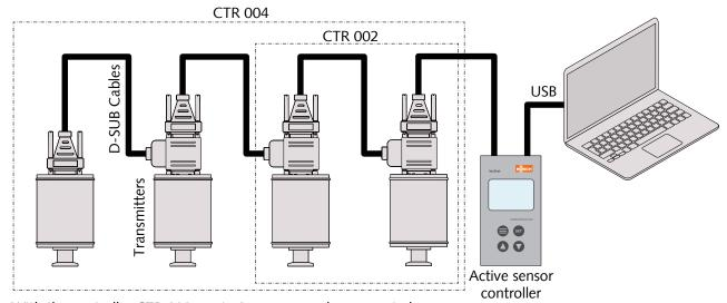
With the controller CTR 002: up to 2 gauges can be connected.
