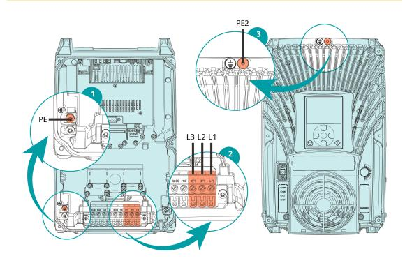
The leakage current exceeds 3.5 mA (AC). According to EN 61800-5-1 an additional protective earth conductor (PE2) must be provided:
