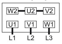
Star connection, multi-voltage motor with 9 pins (high voltage):
