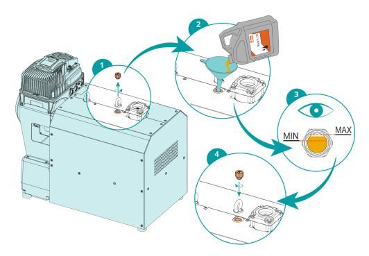
The oil level should stay constant over the lifetime of the oil. If the level does fall, this indicates a leak and the machine requires repair.
