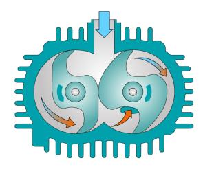
The machine works on the claw principle.
