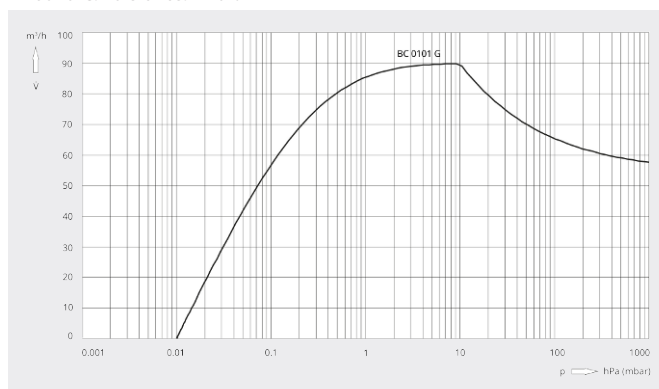
Pumping speed Air at 20°C. Tolerance: \pm 10\%
