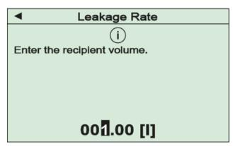
In the next step the internal volume of the vacuum vessel or system has to be entered. After confirmation of the adjusted value by means of the "OK" key the rate-of-rise measurement will be started continuously updating the calculated result for the leakage rate:
