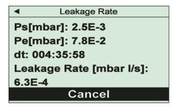
The display shows start pressure Ps, current end pressure Pe, elapsed time dt as well as the calculated leakage rate.
