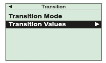
Depending on the selected transition mode you can set the pressure range for a continuous transition or the required pressure for direct switch-over under menu item "Transition Values".
