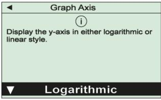
Use this menu item to select whether the y-axis of your plot shall have linear or logarithmic scaling. The setting must finally be confirmed with the "OK"-key.
