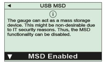
This menu is used to adjust settings of the USB interface and the Bluetooth interface of the VACTEST PPP 700 D.
