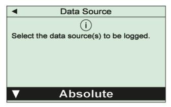
In this menu you can select the data sources for data logging, i.e. if absolute pressure, relative pressure or both should be recorded. The selection must finally be confirmed with the "OK"-key.
