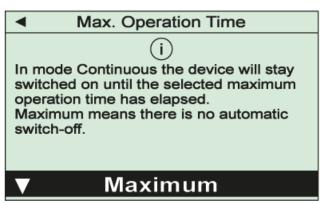
This function assures that the VACTEST PPP 700 D will be switched-off after an adjustable maximum operation time even in operation mode "Continuous". This will avoid unintended discharge of the battery. You can select "Maximum" (no switch-off) and pre-defined time periods between 30 min and 5 h.
