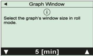
If a rolling mode has been selected as "Graph Mode" this menu item will allow to set the required time frame for the diagram. The setting must finally be confirmed with the "OK"-key.
