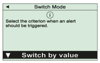
The thresholds to switch-on and switch-off the alert can be edited under menu "Switch Values".
