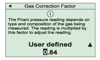
The pressure reading of Pirani sensors depends on type and composition of them gas being measured. The unit is adjusted for  $N_2$  and dry air. For other gases the pressure display can be corrected in the range below 0.5 mbar by multiplication with a related correction factor.
