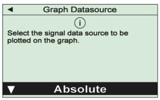
Use this menu item to select the data source for the plot, i.e. absolute or relative pressure. The setting must finally be confirmed with the "OK"-key.
