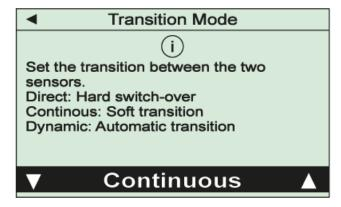
For devices with combination sensors use this menu item to adjust the transition mode between the two sensors:
