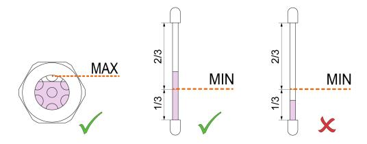
• Fill up if necessary, see Filling Cooling Liquid [→ 18].
