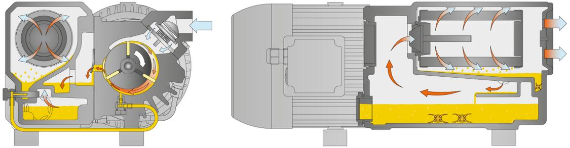
The machine works on the rotary vane principle.
