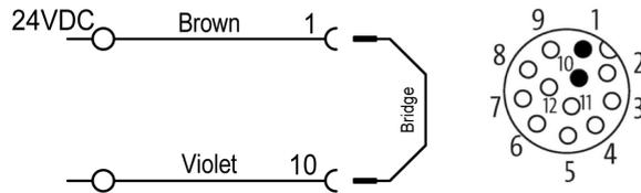
It allows the machine to be started by an external signal.
