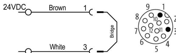
In case of HMI failure, refer to the electrical wiring diagram inside the control unit (CU). The machine then operates at 100% speed and the inlet valve is open.
