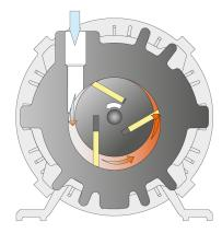
The machine works on the rotary vane principle.
