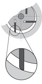
In case the vanes (35) are undamaged, the height A of all vanes is more than 23 mm and regular inspections in short intervals are ensured:
