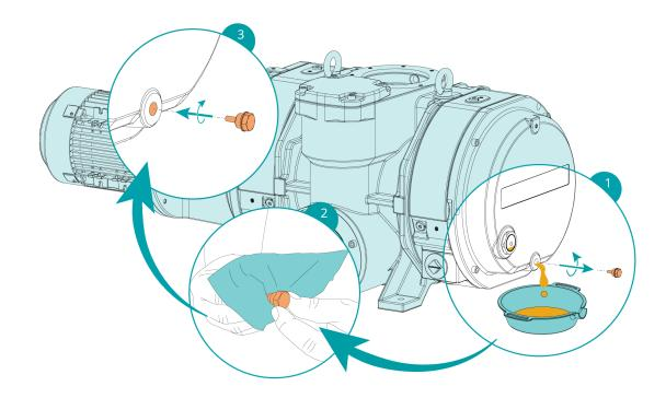
For oil type and oil capacity see Technical Data and Oil [ $\rightarrow$  36].
