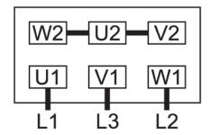
Double star connection, multi-voltage motor with 12 pins (low voltage):
