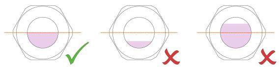
Fill up if necessary, see Filling Cooling Liquid [ $\rightarrow$  22].
