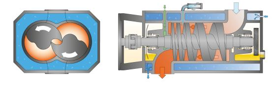
Water-cooled version with plate heat exchanger (optional)
