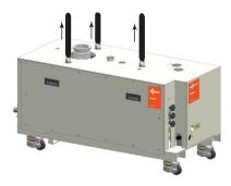
• Unscrew the fixing bolts in the base frame.
