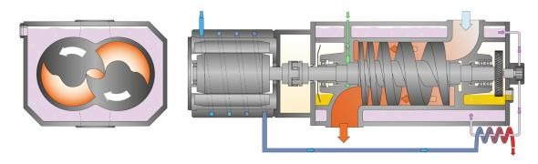
The machine works on the one-stage, twin-screw pump principle.
