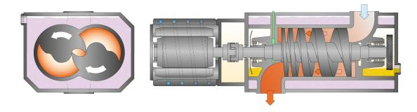
The machine works on the one-stage, twin-screw pump principle.
