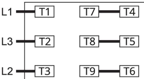
Connection of motor thermistors 3xPTC (recommended):
