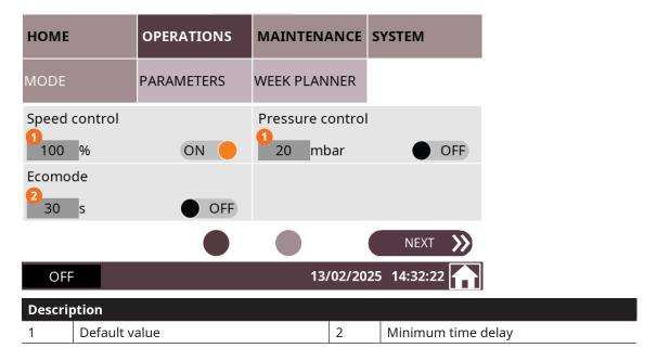
Speed control (Standard). Configured by default with a vacuum pump speed of 100 %, the speed control mode allows the variation of the motor frequency.
