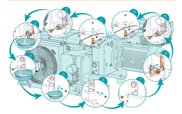
For cooling liquid type and cooling liquid capacity see Technical Data and *Cooling Liquid* [→ 81].
