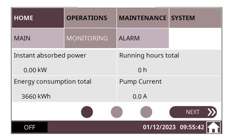
**Instant absorbed power.** Indicates in kW the total absorbed power in real time.
