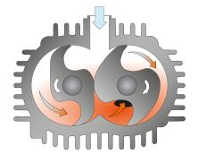
The machine works on the claw principle.
