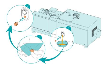
For oil type and oil capacity see *Technical Data* [ $\rightarrow$  29] and *Oil* [ $\rightarrow$  31].
