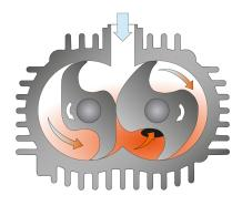
The machine works on the claw principle.
