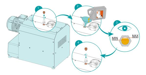
The oil level should stay constant over the lifetime of the oil. If the level does fall, this indicates a leak and the machine requires repair.
