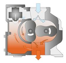
The machine works on the Booster blower principle.
