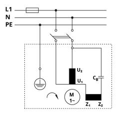
L1 = Phase 1; N = Neutral; PE = Ground  $C_B$  = Capacitor  $M_{1-}$  = Standard single-phase motor  $U_1 - U_2$  = Main phases  $Z_1 - Z_2$  = Auxiliary phases
