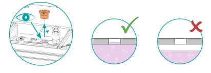
• Fill up if necessary, see Filling Cooling Liquid [ $\rightarrow$  18].
