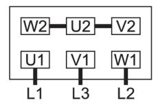
Double star connection, multi-voltage motor with 12 pins (low voltage):
