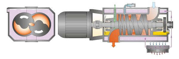
The machine works on the one-stage, twin-screw pump principle.
