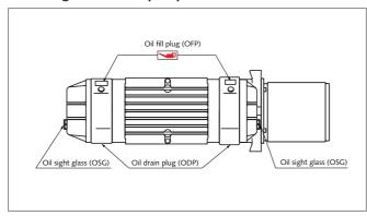
**NOTE:** The quantity of oil specified in the installation handbook is of informative nature only. Check the oil level with the help of the various oil sight glasses (OSG 1, 2, 3) on the vacuum pump.
