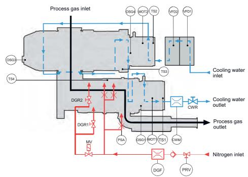
DGF Nitrogen flow meter, dilution gas
