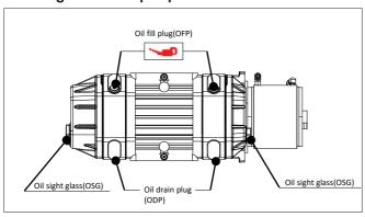
NOTE: The quantity of oil specified in the installation handbook is of informative nature only. Check the oil level with the help of the various oil sight glasses (OSG 1, 2, 3) on the vacuum pump.
