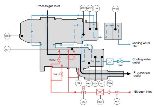
DGF Nitrogen flow meter, dilution gas
