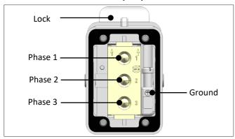
Connect the main cable on the socket, according to the following figure
