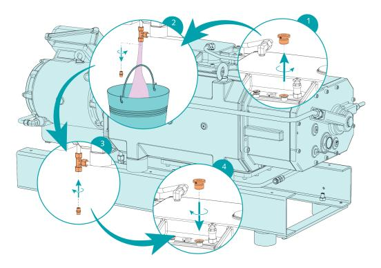
For cooling liquid type and cooling liquid capacity see Technical Data and *Cooling Liquid* [ $\rightarrow$  38].
