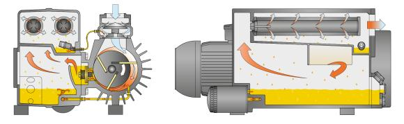
The machine works on the rotary vane principle. The oil seals the gaps, lubricates the vanes and takes away compression heat. The oil filter cleans the circulating oil. Exhaust filters separate the oil from the discharged gas.
