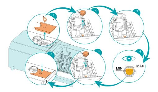
The oil level should stay constant over the lifetime of the oil. If the level does fall, this indicates a leak and the machine requires repair.
