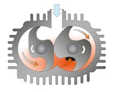
The machine works on the claw principle.
