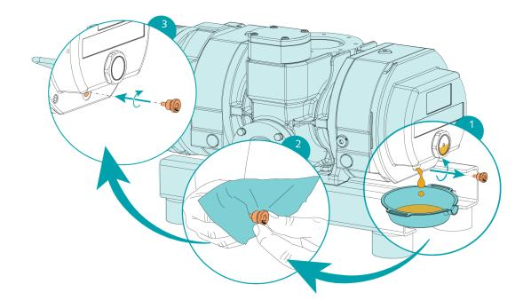
For oil type and oil capacity see *Technical Data* [ $\rightarrow$  30] and *Oil* [ $\rightarrow$  31].
