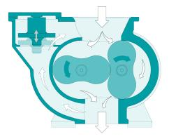
The machine works on the Booster blower principle. The two oil housings (on each side) allow the lubrication of the gears and bearings. A bypass valve (BPV) limits automatically the differential pressure between inlet and outlet.
