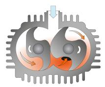
The machine works on the claw principle.
