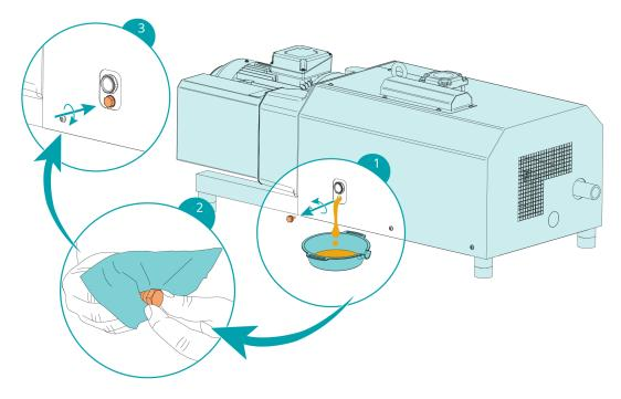
For oil type and oil capacity see *Technical Data* [ $\rightarrow$  27] and *Oil* [ $\rightarrow$  28].
