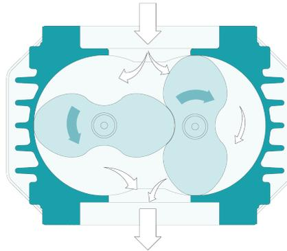
The machine works on the Booster blower principle.
