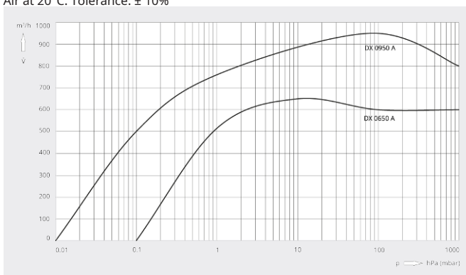
Pumping speed Air at 20°C. Tolerance: \pm 10\%
