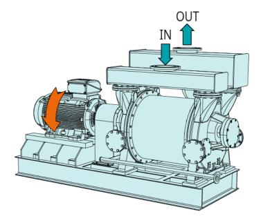
• Watch the fan wheel of the motor and determine the direction of rotation just before the fan wheel stops.
