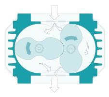
The machine works on the Booster blower principle.
