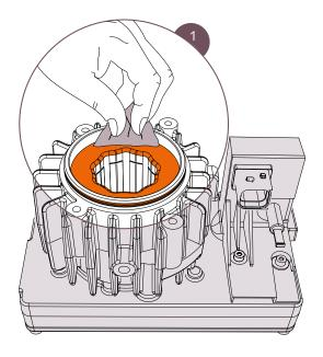
• 2. Remove the existing O-Ring carefully to avoid damaging the groove.
