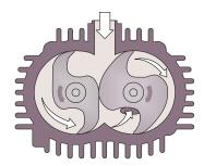
The machine works on the claw principle.
