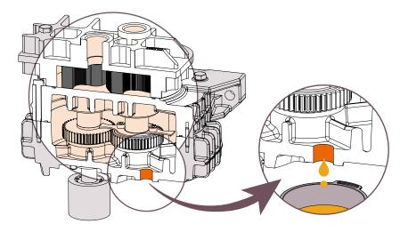
• The illustration below shows the "vertical position" for oil refilling.
