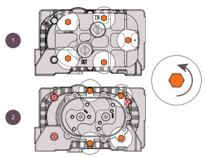
• 2. Then remove the four M6 screws holding the motor. Do not unscrew the 3 other screws!
