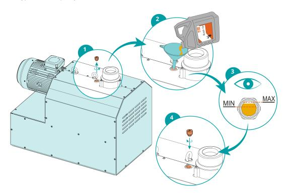
The oil level should stay constant over the lifetime of the oil. If the level does fall, this indicates a leak and the machine requires repair.
