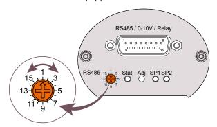
The communication is effected via serial interface RS485:
