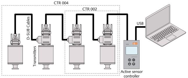
With the controller CTR 002: up to 2 gauges can be connected. With the controller CTR 004: up to 4 gauges can be connected.
