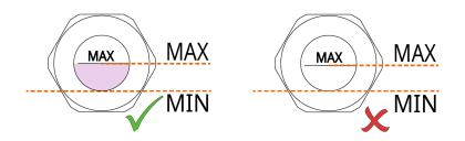
• Fill up if necessary, see Filling Cooling Liquid [ $\rightarrow$  19].
