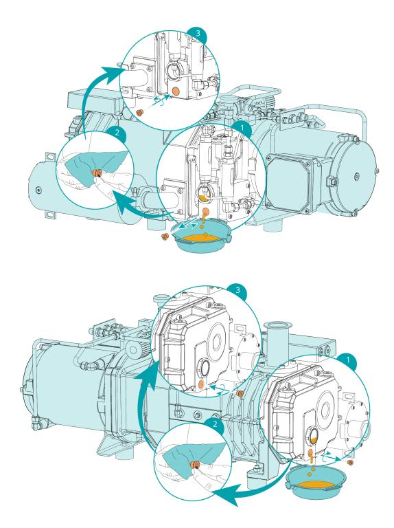
For oil type and oil capacity see Technical Data and *Oil* [ $\rightarrow$  41].
