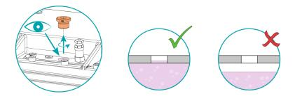
• Fill up if necessary, see Filling Cooling Liquid [→ 19].
