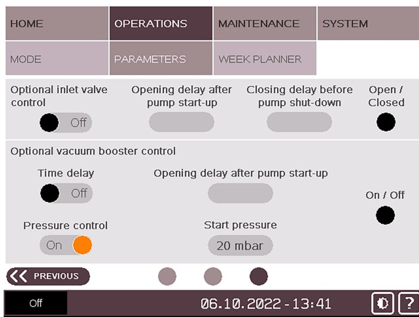
The booster start signal is given by the PLUS pump when the pressure reaches a set value (Default value 20 mbar).
