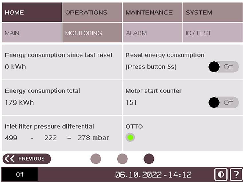
**Energy consumption since last reset:** Indicates the energy consumption in kWh since the last reset.
