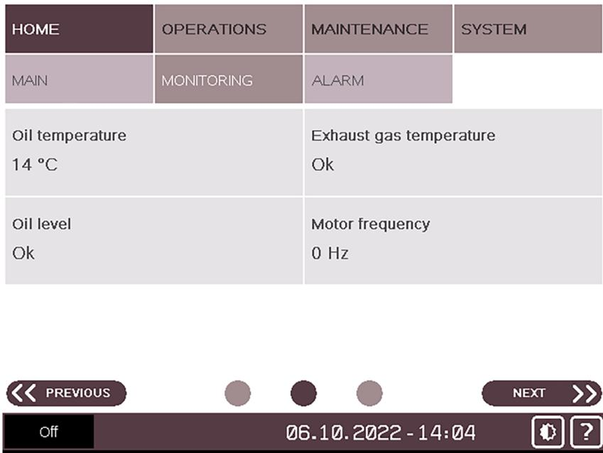
**Oil temperature:** Indicates the oil temperature, in case of a too high temperature a warning or an alarm occurs, see *Dysfunction* [→ 55].
